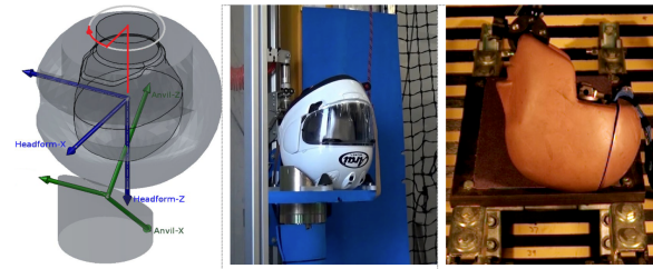
Composite Figure 20: Oblique Impact Test for rTBI
