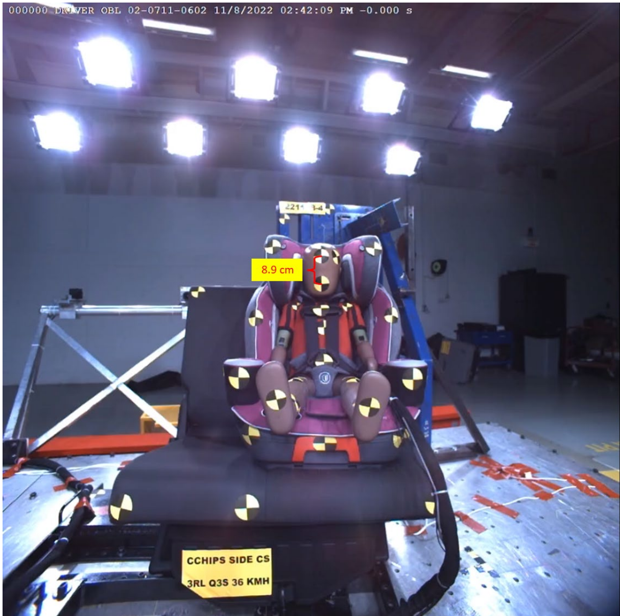
Figure B3: The measured distance between the camera targets on the Q3s's forehead and chin (8.9 cm) was used to calibrate the frontal-view videos for each far-side impact with the Q3s. These camera targets were not moved or removed across all tests with the Q3s.
