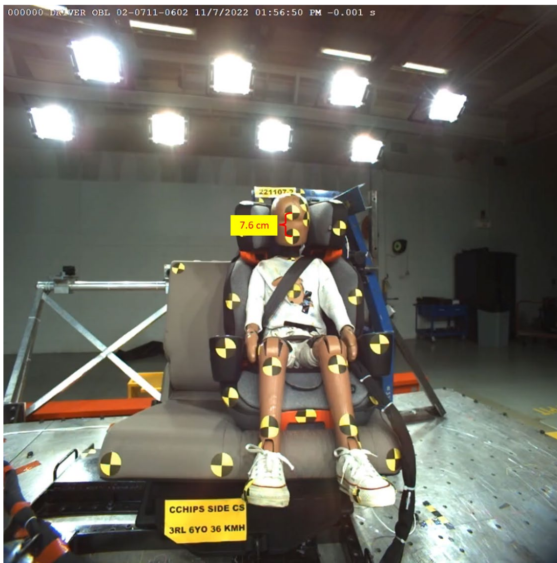
Figure B2: The measured distance between the camera targets on the Hybrid III 6yo's forehead and chin (7.6 cm) was used to calibrate the frontal-view videos for each far-side impact with the Hybrid III 6yo. These camera targets were not moved or removed across all tests with the Hybrid III 6yo.
