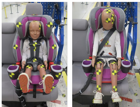
Figure 2: Pre-test positions of the 3yo Hybrid III in FF harness CRS 1 (left) and Hybrid III 6yo in Booster 1 (right).
