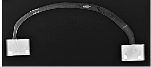
Figure F13. Pair 13 rib (left) and rib+CC (right) post-test x-rays (not to scale)
