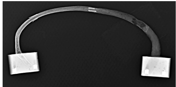
Figure F2. Pair 2 rib (left) and rib+CC (right) post-test x-rays (not to scale)
