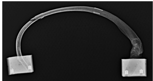
Figure F4. Pair 4 rib (left) and rib+CC (right) post-test x-rays (not to scale)
