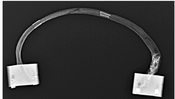
Figure F15. Pair 15 rib (left) and rib+CC (right) post-test x-rays (not to scale)
