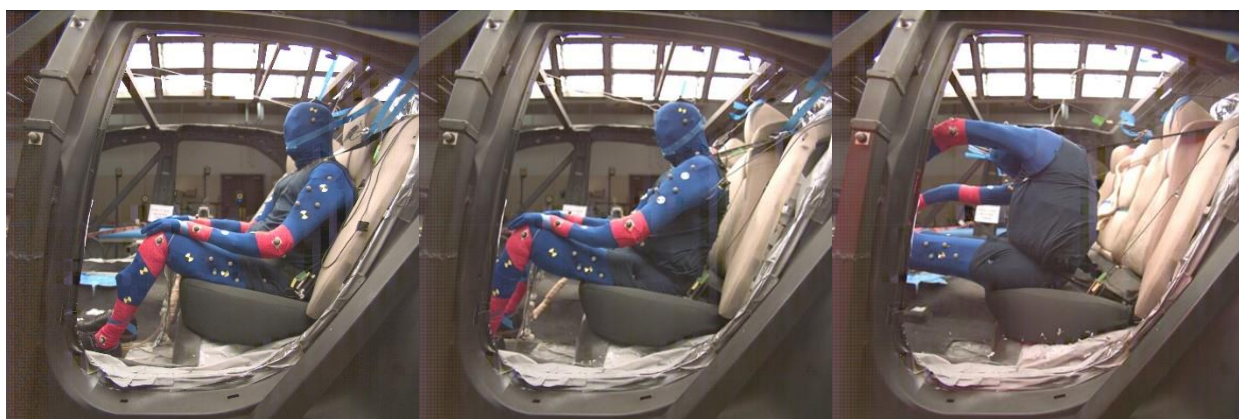
FIGURE D15. Images for test V19-6 at the start of the test (left), at the midpoint of forward excursion (middle), and time of peak excursion (right).
