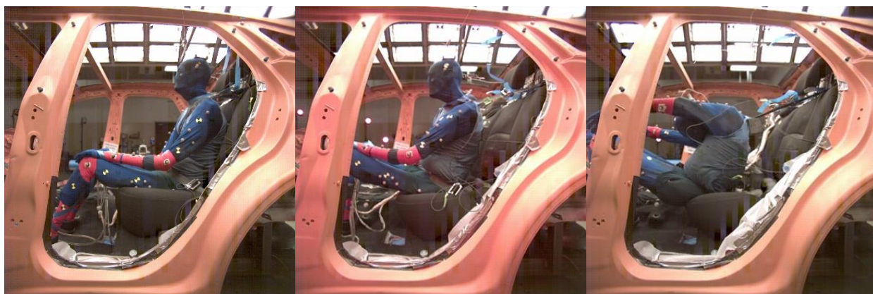
FIGURE D2. Images for test V13-4 at the start of the test (left), at time of submarining (middle), and time of peak excursion (right).
