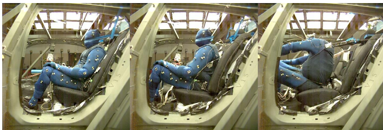
FIGURE D12. Images for test V15-7 at the start of the test (left), at time of pelvis fracture (middle), and time of peak excursion (right).
