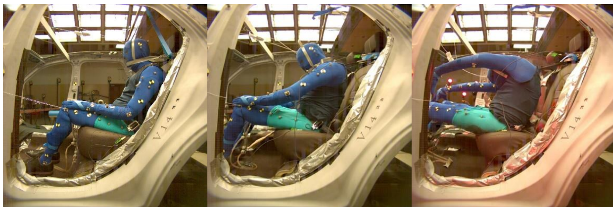
FIGURE D7. Images for test V14-6 at the start of the test (left), at time of submarining (middle), and time of peak excursion (right).
