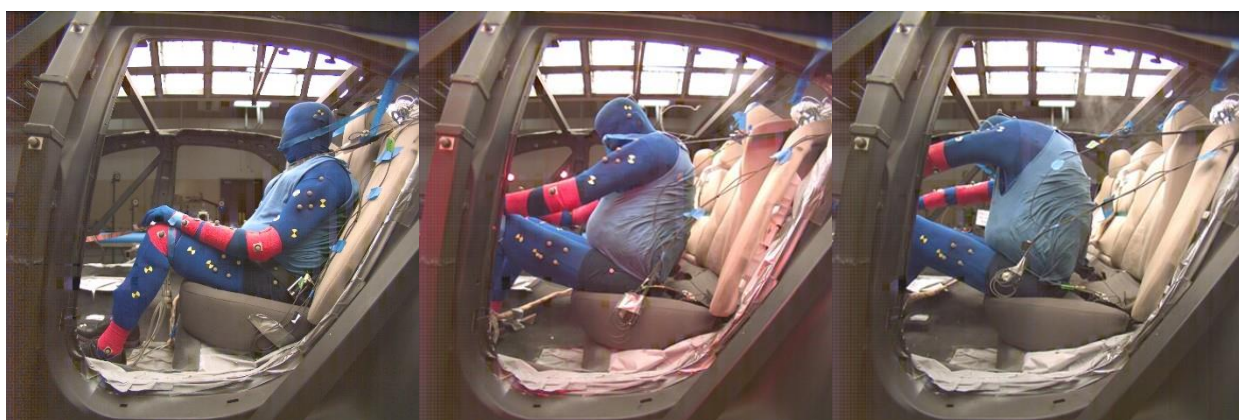
FIGURE D14. Images for test V19-5 at the start of the test (left), at time of pelvis fracture (middle), and time of peak excursion (right).
