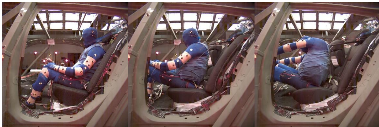
FIGURE D10. Images for test V15-5 at the start of the test (left), at time of pelvis fracture (middle), and time of peak excursion (right).
