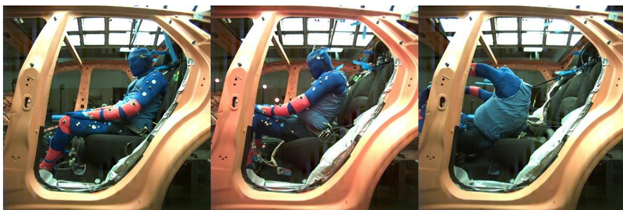
FIGURE D3. Images for test V13-5 at the start of the test (left), at time of submarining (middle), and time of peak excursion (right).
