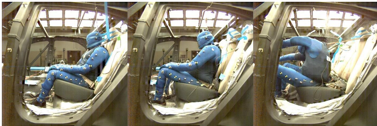
FIGURE D16. Images for test V19-7 at the start of the test (left), at the midpoint of forward excursion (middle), and time of peak excursion (right).
