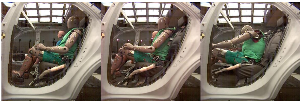
FIGURE D5. Images for test V14-4 at the start of the test (left), midpoint of forward excursion (middle), and time of peak excursion (right).
