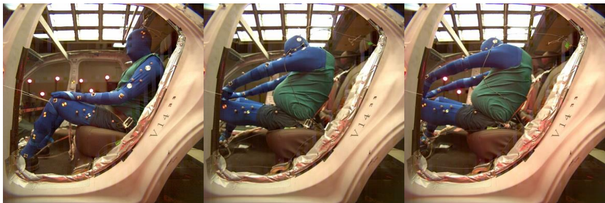
FIGURE D6. Images for test V14-5 at the start of the test (left), at time of pelvis fracture (middle), and time of peak excursion (right).
