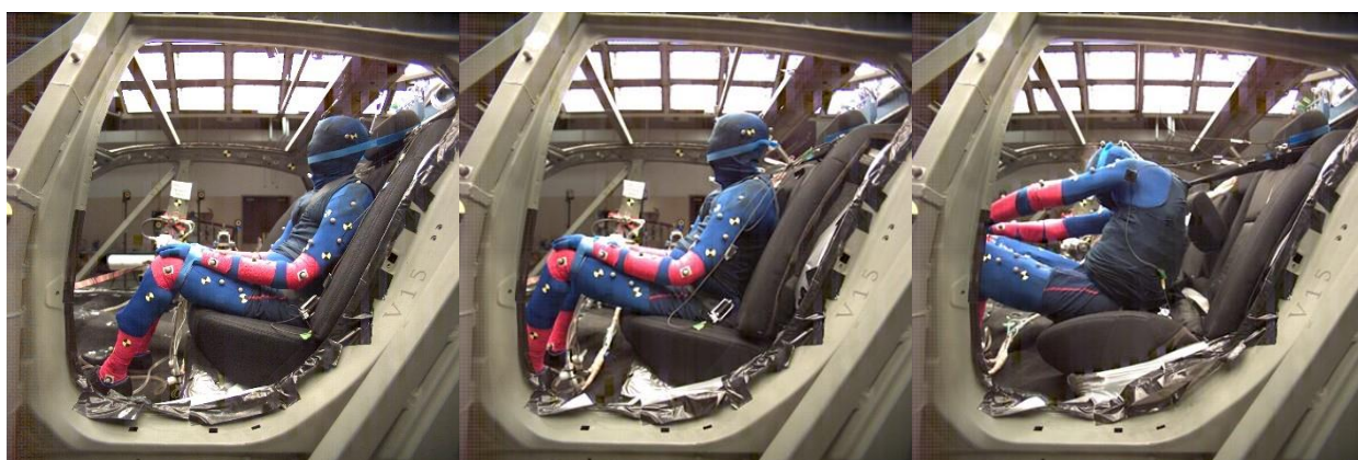
FIGURE D11. Images for test V15-6 at the start of the test (left), at the midpoint of forward excursion (middle), and time of peak excursion (right).
