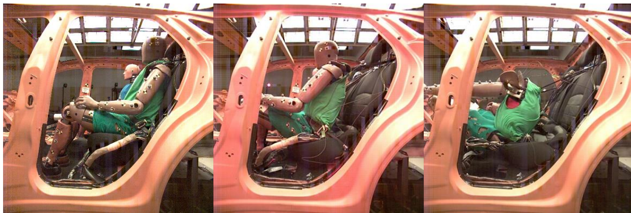
FIGURE D1. Images for test V13-2 at the start of the test (left), at time of submarining (middle), and time of peak excursion (right).
