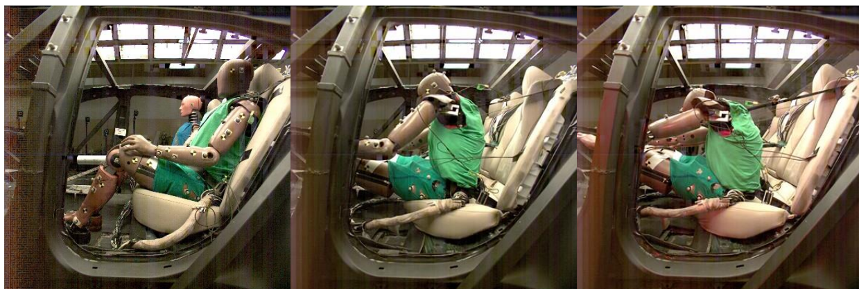
FIGURE D13. Images for test V19-4 at the start of the test (left), at time of submarining (middle), and time of peak excursion (right).
