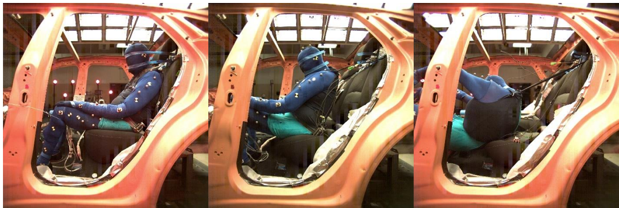
FIGURE D4. Images for test V13-6 at the start of the test (left), at time of submarining (middle), and time of peak excursion (right).
