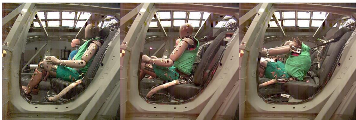
FIGURE D9. Images for test V15-4 at the start of the test (left), at time of submarining (middle), and time of peak excursion (right).
